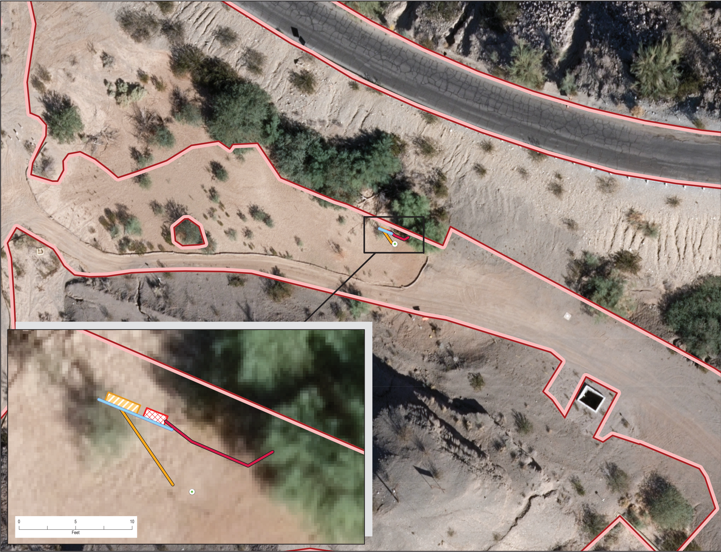
FIGURE 1 Proposed Relocation of Power/Control Equipment to Aboveground at IRZ-39 Work Variance Request #13 PG&E Topock Compressor Station Needles, California
