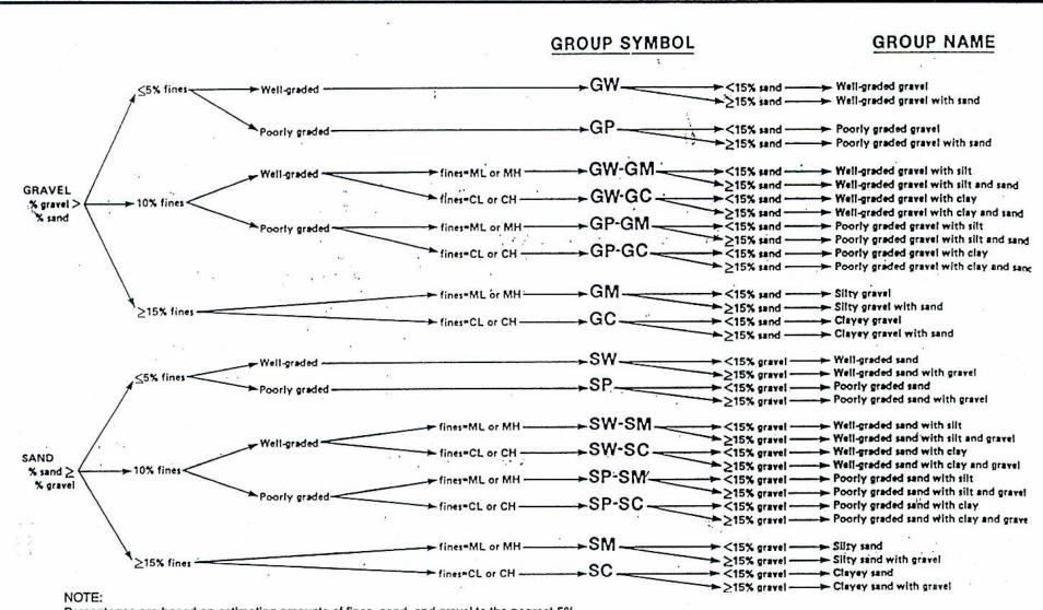
Percentages are based on estimating amounts of fines, sand, and gravel to the nearest 5% (After ASTM Designation D2488 Standard Test Method for Classification of Solls for Engineering Purposes)
