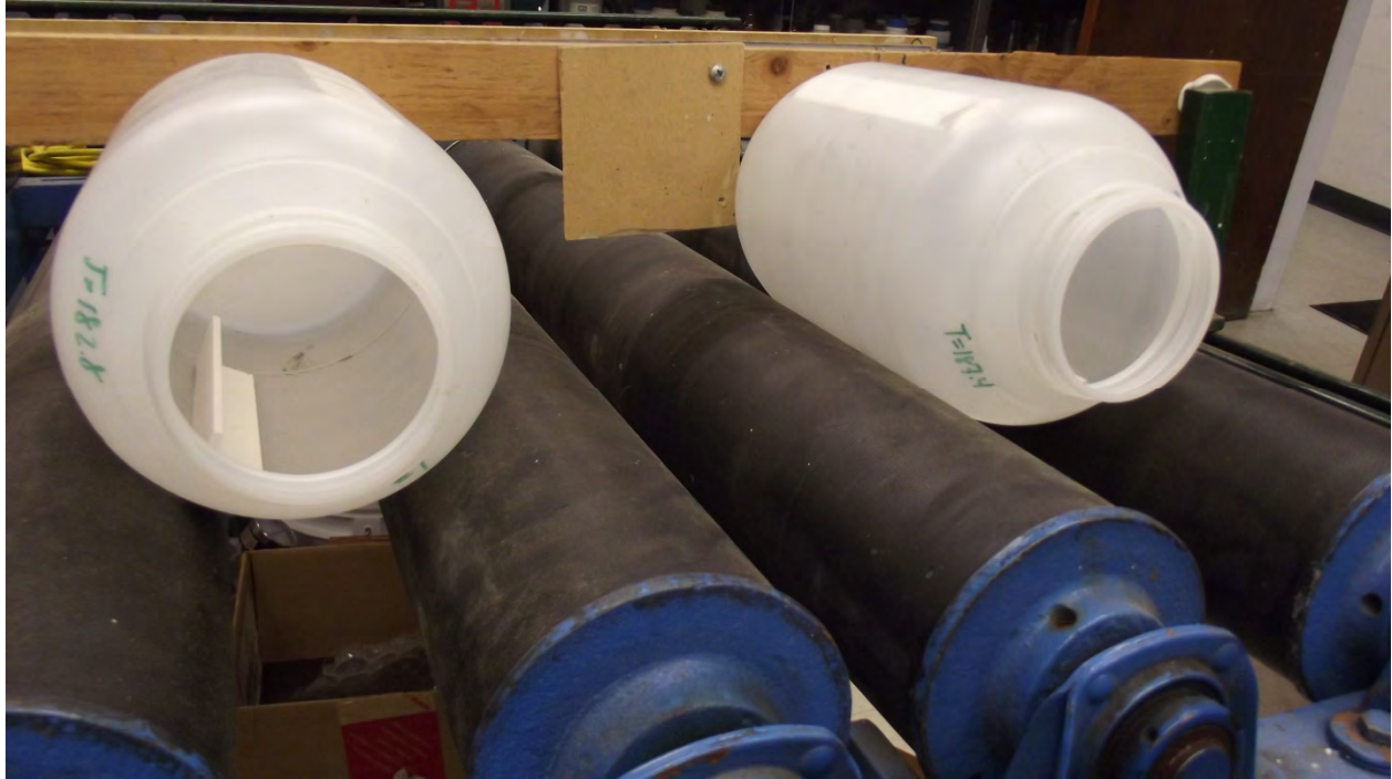
Figure 3. Batch Trommel Soil Washing Equipment Setup
