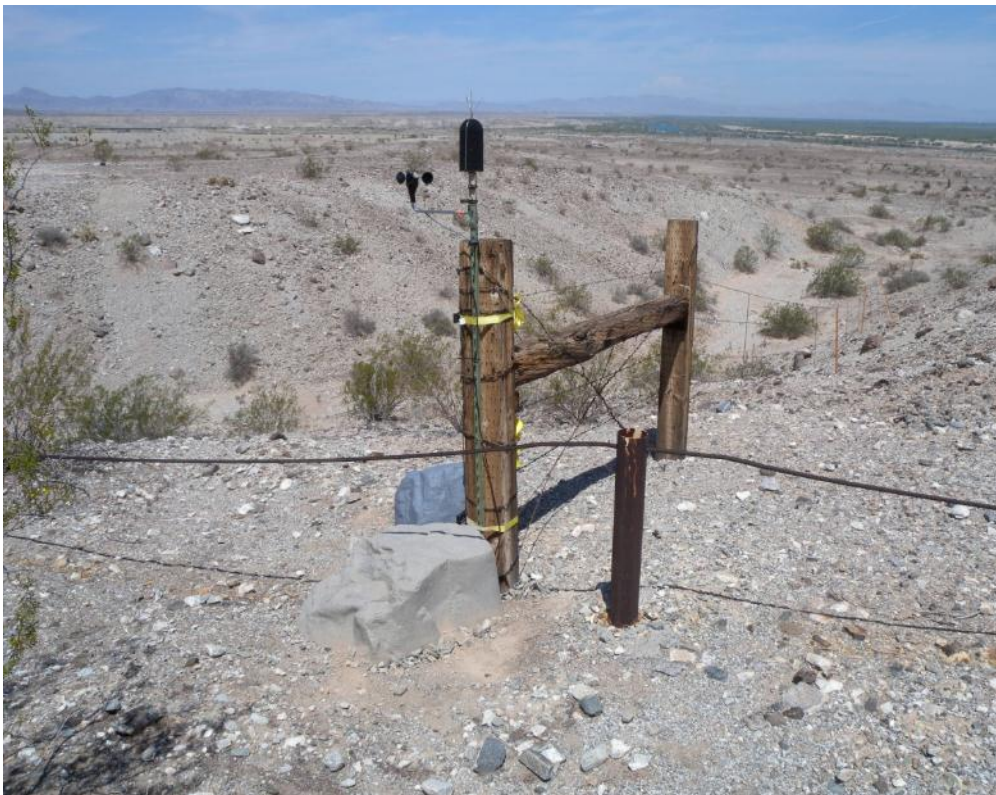
Photograph 2: Temporary Noise Monitoring Station set up in proximity to ST-1 noise measurement location in the certified EIR (DTSC, 2011), taken August 2012.
