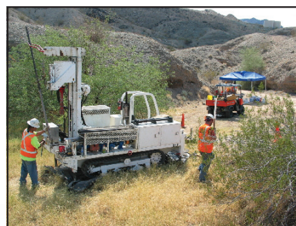
Soil Sampling with Direct Push Drill Rig
