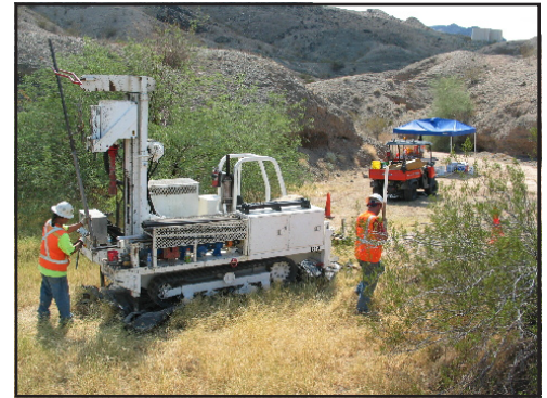
Soil Sampling with Direct Push Drill Rig
