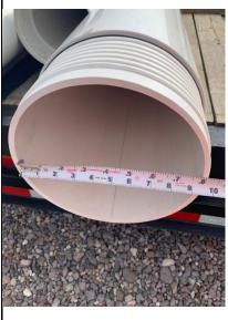
8/20/2022 – TWB-03: 10-inch Shur-Grip SDR-17 PVC casing with an inner diameter of 0.79 feet
