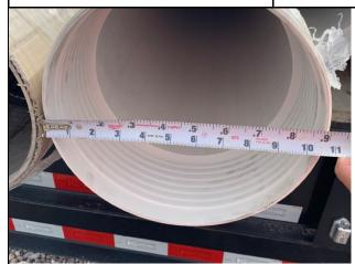
8/20/2022 – TWB-03: 10-inch Shur-Grip SDR-17 PVC casing with an outer diameter of 0.89 feet
