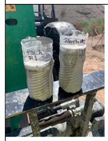
8/23/2022 - TWB-03: Grout cured from batch #1 and #2
