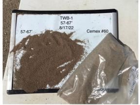
Core Depth: 57 to 67 Sand removed by overdrilling Date: 8/17/2022
