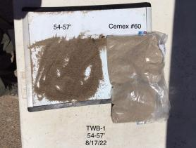
Core Depth: 54 to 57 Description: Cemex #60 (40x70) Lapis Lustre Description: Cemex #60 (40x70) Lapis Lustre Sand Description: Cemex #60 (40x70) Lapis Lustre removed by overdrilling Date: 8/17/2022
