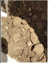
Core Depth: 34 to 44 Description: Cemex #60 (40x70) Lapis Lustre Sand removed by overdrilling Date: 8/16/2022
