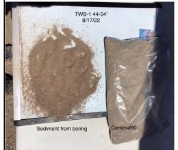
Core Depth: 44 to 54 Sand removed by overdrilling Date: 8/17/2022
