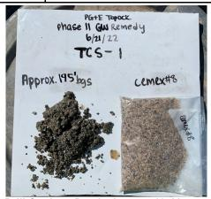
Drill Cuttings Depth: Approx. 195' bgs Description: Confirmation of Cemex 8 Mesh Lapis Lustre Sand in drill cuttings.
