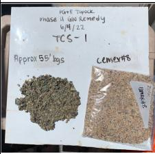
Drill Cuttings Depth: Approx. 55' bgs Description: Confirmation of Cemex 8 Mesh Lapis Lustre Sand in drill cuttings. Date: 6/4/2022
