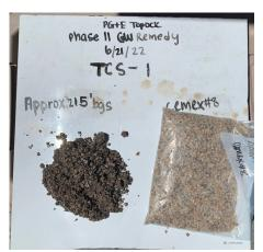
Drill Cuttings Depth: Approx. 215' bgs Description: Confirmation of Cemex 8 Mesh Lapis Lustre Sand in drill cuttings.
