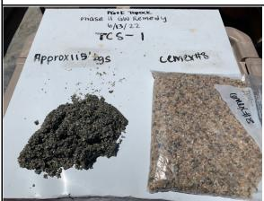
Drill Cuttings Depth: Approx. 115' bgs Description: Confirmation of Cemex 8 Mesh Lapis Description: Confirmation of Cemex 8 Lustre Sand in drill cuttings.
