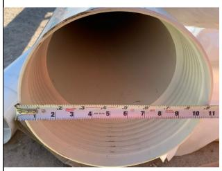
6/24/2022 – TCS-01: 10-inch Shur-Grip SDR-17 PVC casing outer diameter (10.80-inches)
