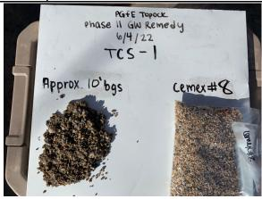
Drill Cuttings Depth: Approx. 10' bgs Description: Confirmation of Cemex 8 Mesh Lapis Description: Confirmation of Cemex 8 Mesh Lustre Sand in drill cuttings.
