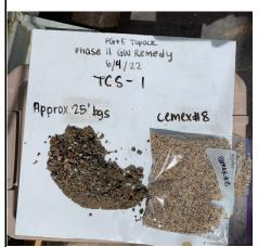
Drill Cuttings Depth: Approx. 25' bgs Description: Confirmation of Cemex 8 Mesh Lapis Lustre Sand in drill cuttings. Date: 6/4/2022
