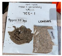
Drill Cuttings Depth: Approx. 35' bgs Description: Confirmation of Cemex 8 Mesh Lapis Description: Confirmation of Cemex 8 Mesh Lustre Sand in drill cuttings.
