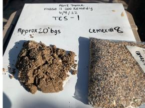
Drill Cuttings Depth: Approx. 20' bgs Lapis Lustre Sand in drill cuttings.
