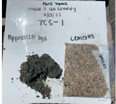
Drill Cuttings Depth: Approx. 125' bgs Mesh Lapis Lustre Sand in drill cuttings.
