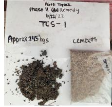
Drill Cuttings Depth: Approx. 245' bgs Description: Confirmation of Cemex 8 Mesh
