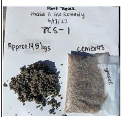
Drill Cuttings Depth: Approx. 145' bgs Description: Confirmation of Cemex 8 Mesh Lapis Description: Confirmation of Cemex 8 Lustre Sand in drill cuttings.
