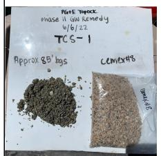
Drill Cuttings Depth: Approx. 85' bgs Description: Confirmation of Cemex 8 Mesh Lapis Lustre Sand in drill cuttings. Date: 6/6/2022
