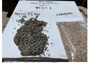
**Drill Cuttings Depth: Approx. 75' bgs** Description: Confirmation of Cemex 8 Mesh Lapis Description: Confirmation of Cemex 8 Mesh Lapis Lustre Sand in drill cuttings. Date: 6/6/2022
