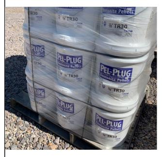
6/29/2022 – TCS-01: Pel-Plug Bentonite Pellets 3/8" TR30 used for intermediate seal
