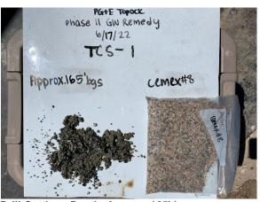
Drill Cuttings Depth: Approx. 165' bgs **Description: Confirmation of Cemex 8 Mesh Lapis**
