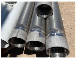
6/24/2022 - TCS-01: 10-inch 18-slot, 316L Stainless Steel Wire Wrap Screen
