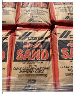
6/26/2022 – TCS-01: Cemex #1/20 Mesh (20x40) Lapis Lustre Sand used for upper and lower filter pack
