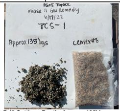
Drill Cuttings Depth: Approx. 135' bgs **Description: Confirmation of Cemex 8 Mesh Lapis**
