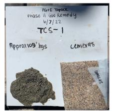
Drill Cuttings Depth: Approx. 105' bgs Lustre Sand in drill cuttings.
