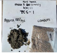
Drill Cuttings Depth: Approx. 185' bgs Description: Confirmation of Cemex 8 Mesh Lapis Lustre Sand in drill cuttings.
