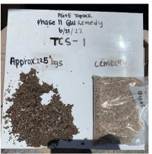
Drill Cuttings Depth: Approx. 225' bgs Description: Confirmation of Cemex 8 Mesh Lapis Lustre Sand in drill cuttings.
