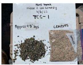
Drill Cuttings Depth: Approx. 95' bgs Description: Confirmation of Cemex 8 Mesh Lapis Description: Confirmation of Cemex 8 Mesh Lapis Lustre Sand in drill cuttings. Date: 6/6/2022
