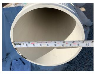
6/24/2022 – TCS-01: 10-inch Shur-Grip SDR-17 PVC casing inner diameter (9.24-inch)
