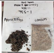
Drill Cuttings Depth: Approx. 255' bgs Description: Confirmation of Cemex 8 Mesh
