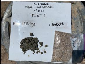
Drill Cuttings Depth: Approx. 175' bgs Description: Confirmation of Cemex 8 Mesh Lapis
