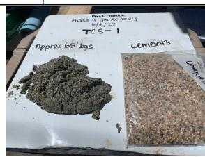
Drill Cuttings Depth: Approx. 65' bgs Lustre Sand in drill cuttings.
