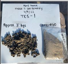
Drill Cuttings Depth: Approx. 3' bgs Description: Confirmation of Cemex #60 Lapis Lustre Sand in drill cuttings.
