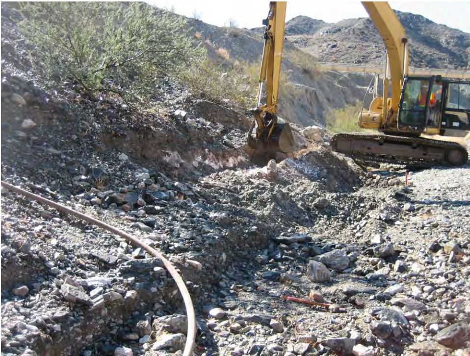
Photograph 22: Horizontal lens of white powder in small observation trench located between trenching locations SWMU1-WP-6a and SWMU1-WP-7
