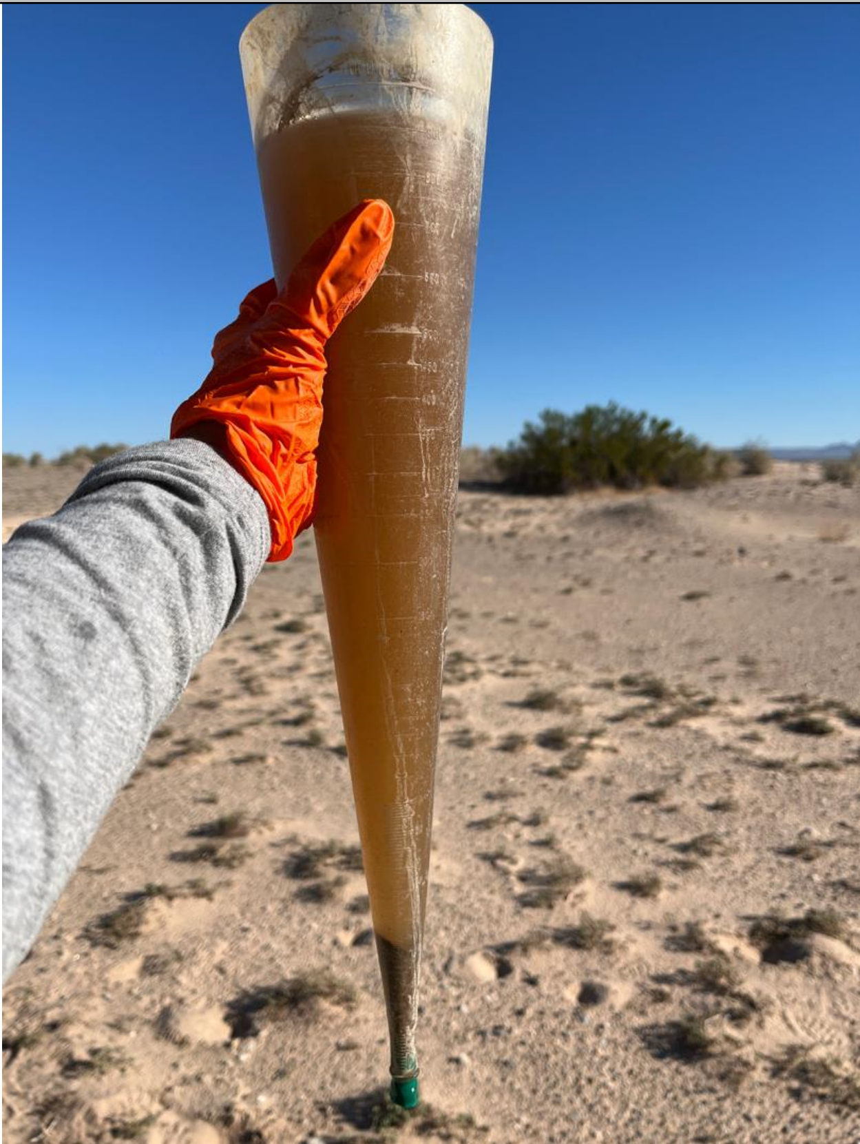
MW-77-046- Water and sediment removed by first bailer, first round of bailing.
