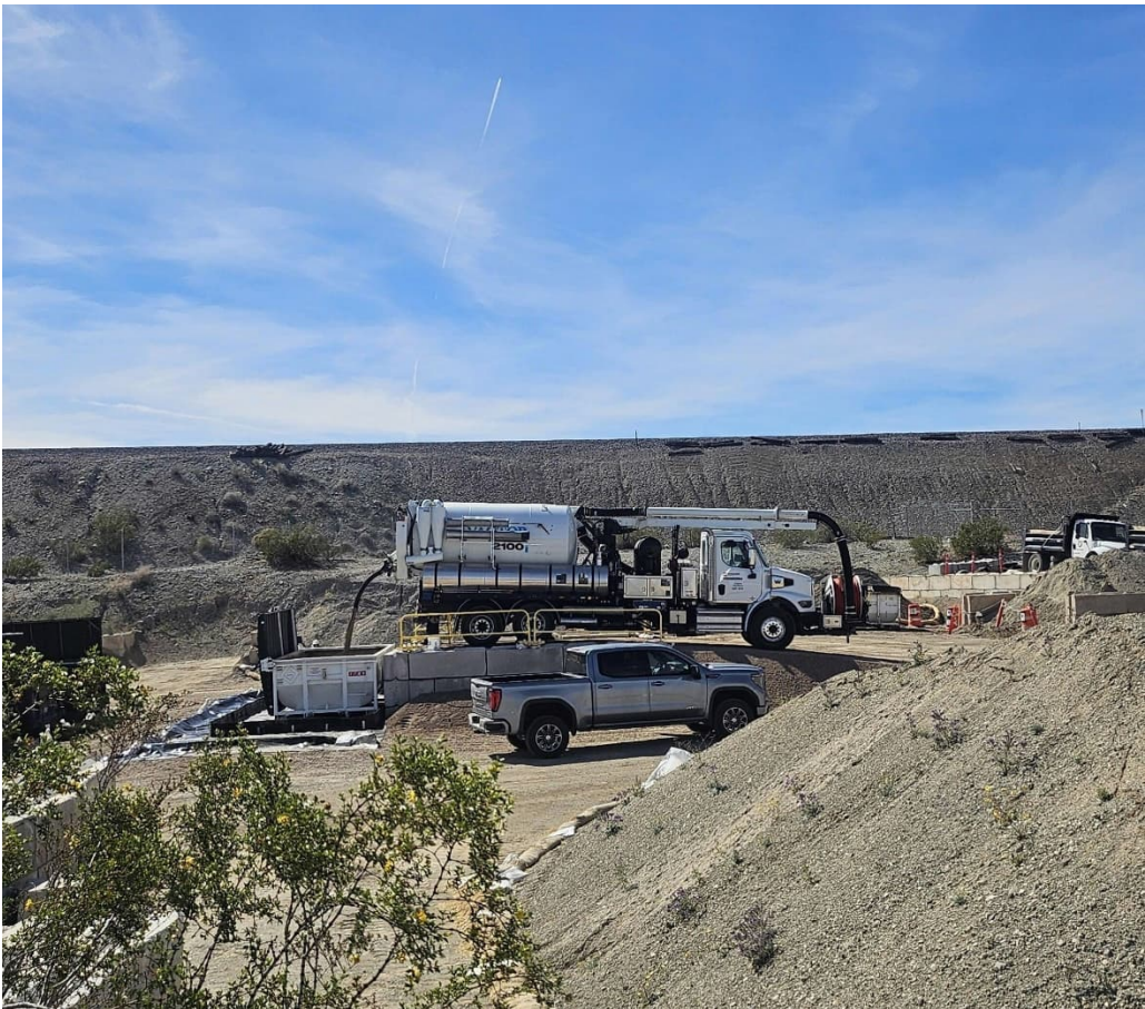
Photo showing a vac truck offloading IRL-01 drilling wastewater into a roll off bin.
