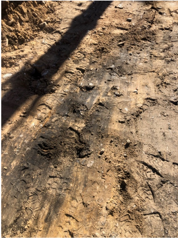
Photo showing a stained soil stripe encountered during excavation near the northwest corner of the carbon amendment footprint on the MW-20 Bench. An opportunistic sample of the stained soil was collected on December 17, 2019.
