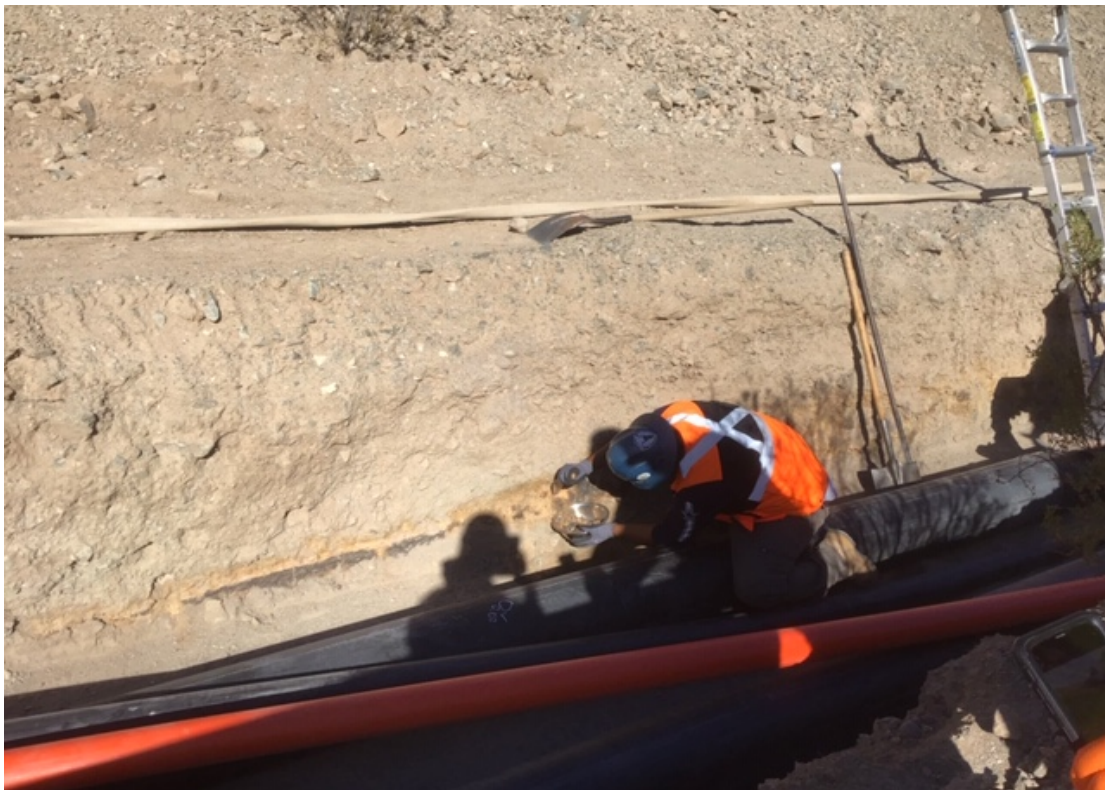
Photo showing sampling of stained soil encountered at Pipeline B.
