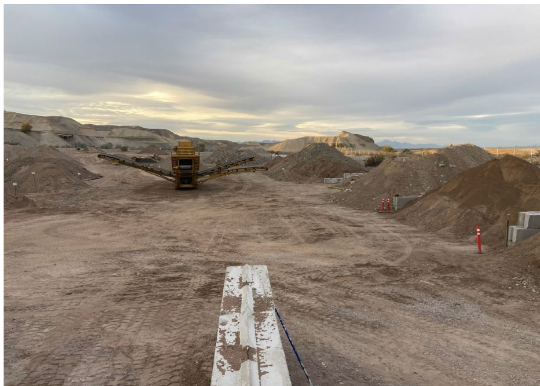
Photo showing the soil sorting machine at the Soil Processing Yard (SPY). The sorted soil piles are placed into stalls that are built along the perimeter of the yard.
