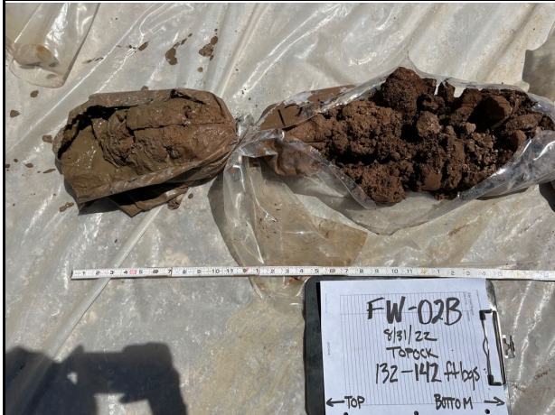
Core Depth: 132 to 142 ft bgs Description: First bag approx. 132 to 134.5 ft bgs, second bag approx. 134.5 to 137 ft bgs Date: 8/31/2022
