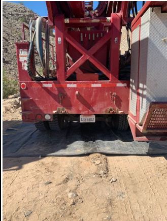
Core Depth: 0 Description: DR Rig centered over pilot borehole. Date: 10/12/2022
