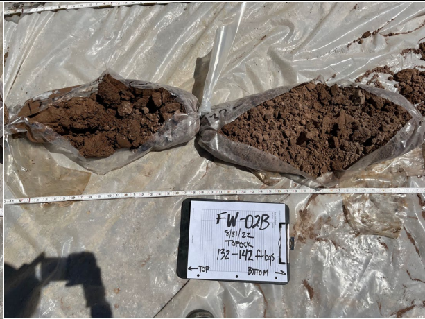
Core Depth: 132 to 142 ft bgs Description: First bag approx. 134.5 to 137 ft bgs, second bag approx. 137 to 139.5 ft bgs. Date: 8/31/2022
