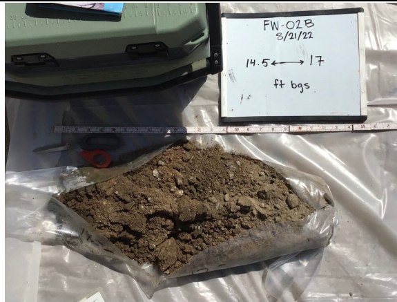
Core Depth: 8 to 10.5 ft bgs Description: Depths on wipe board are not correct. Date: 8/21/2022
