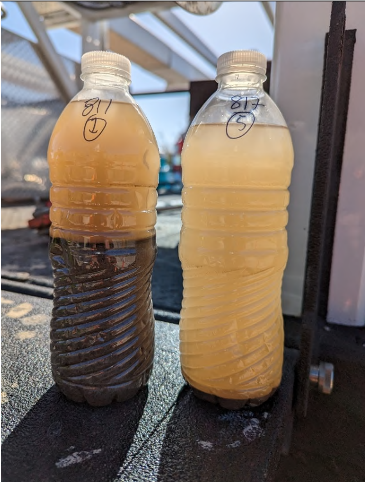
Results of second round of bailing, which occurred on 5/13/2023. Left bottle shows first bailer removed and right bottle shows last bailer of the round which ended up being the 5th bail. Second redevelopment day.
