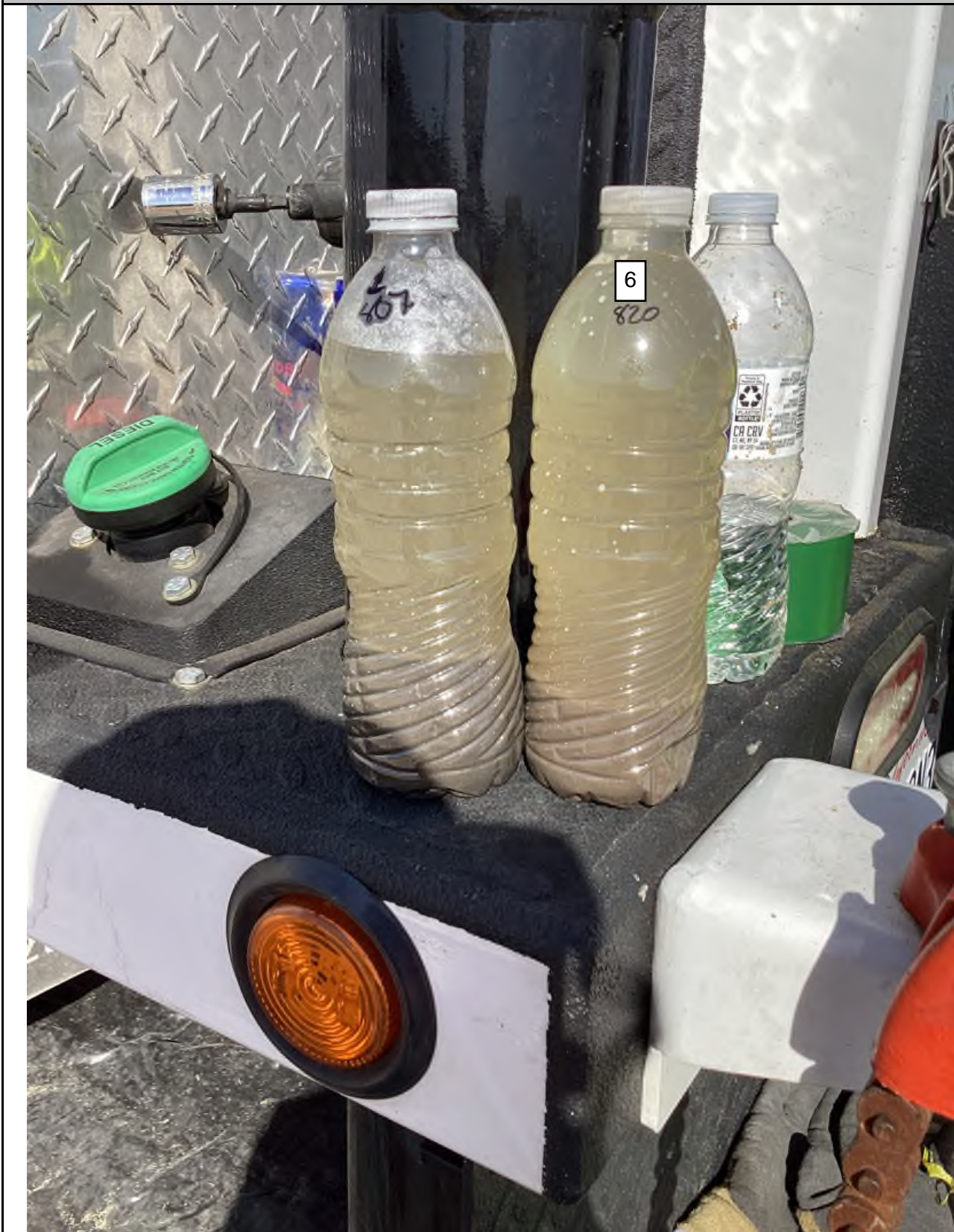
Results of first round of bailing on 5/11/2023. Left bottle shows first bailer removed and right bottle shows last bailer of the round which was the 6th bail. First redevelopment day.
