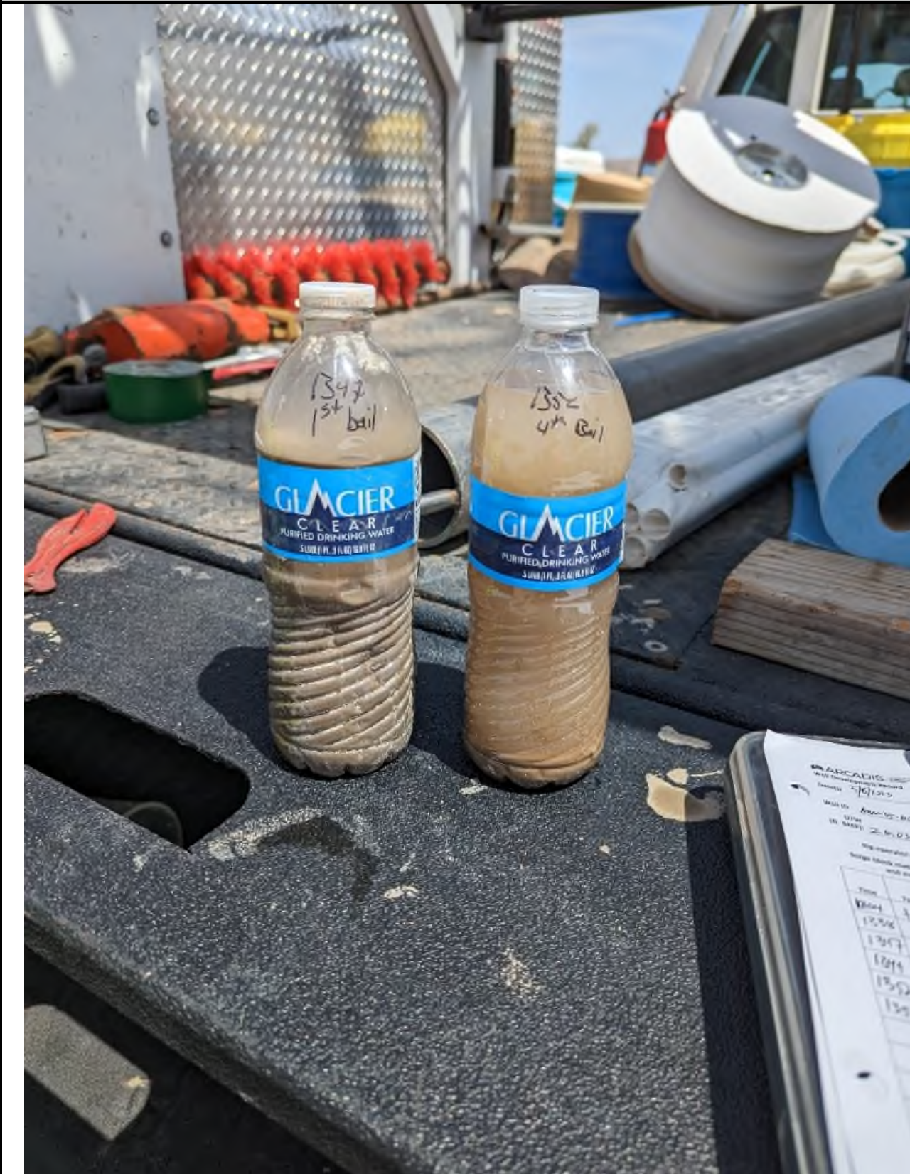
Results of first round of bailing on 5/9/2023. Left bottle shows first bailer removed and right bottle shows last bailer of the round which ended up being the 4th bail. First redevelopment day.
