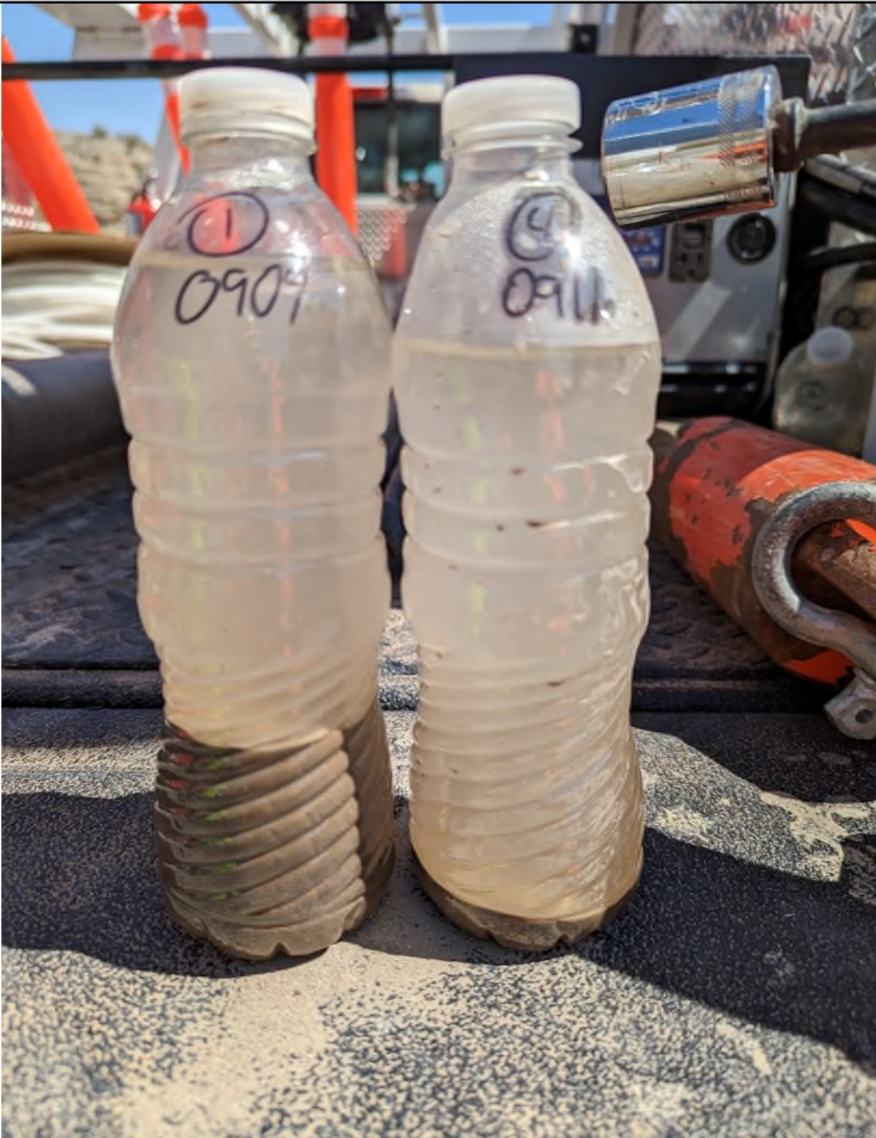
Results of first round of bailing. Left bottle shows first bailer removed and right bottle shows last bailer of the round which was the 4th bail.
