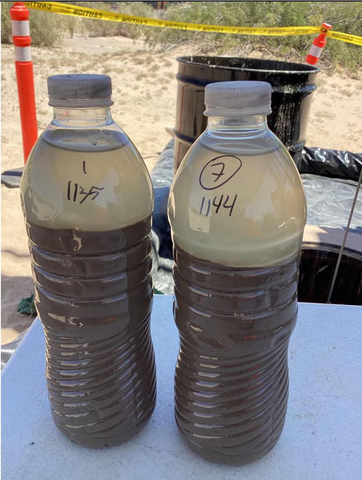
Results of second round of bailing on 5/11/2023. Left bottle shows first bailer removed and right bottle shows last bailer of the round which was the 7th bail. First redevelopment day.
