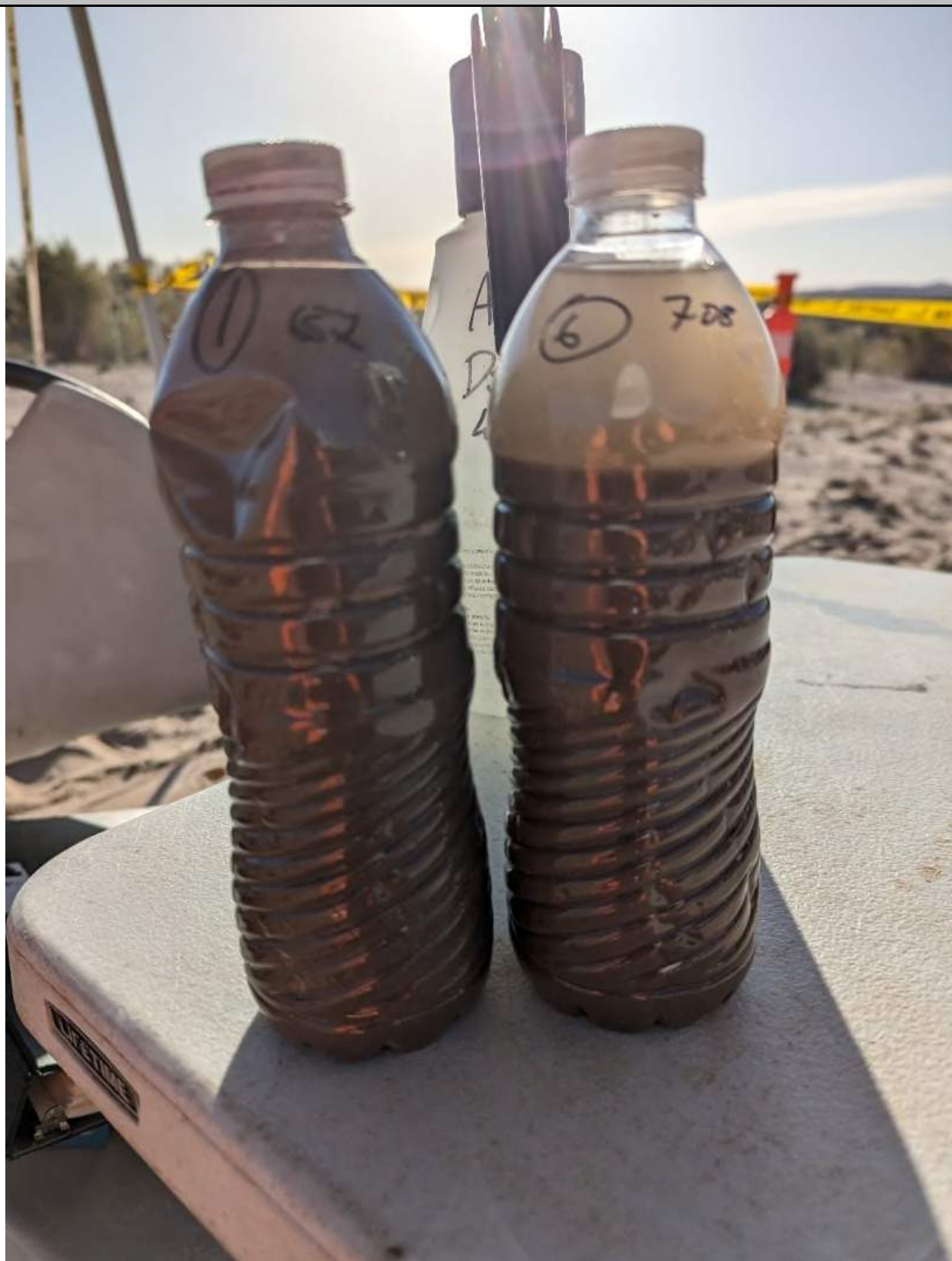
Results of fourth round of bailing on 5/12/21. Left bottle shows first bailer removed and right bottle shows last bailer of the round which was the 6th bail. Second redevelopment day.
