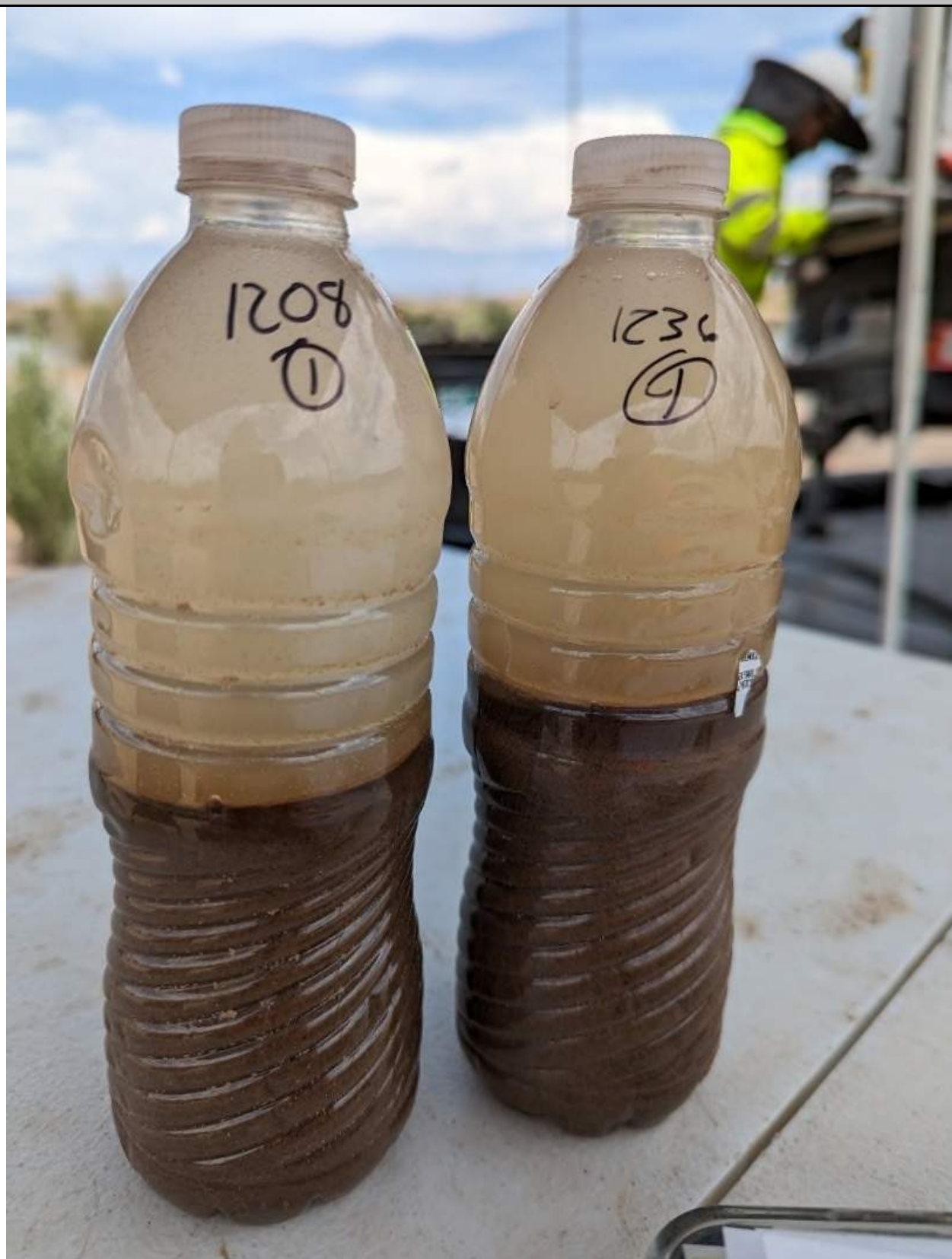
Results of second round of bailing, which occurred on 5/16/23. Left bottle shows first bailer removed and right bottle shows last bailer of the round.
