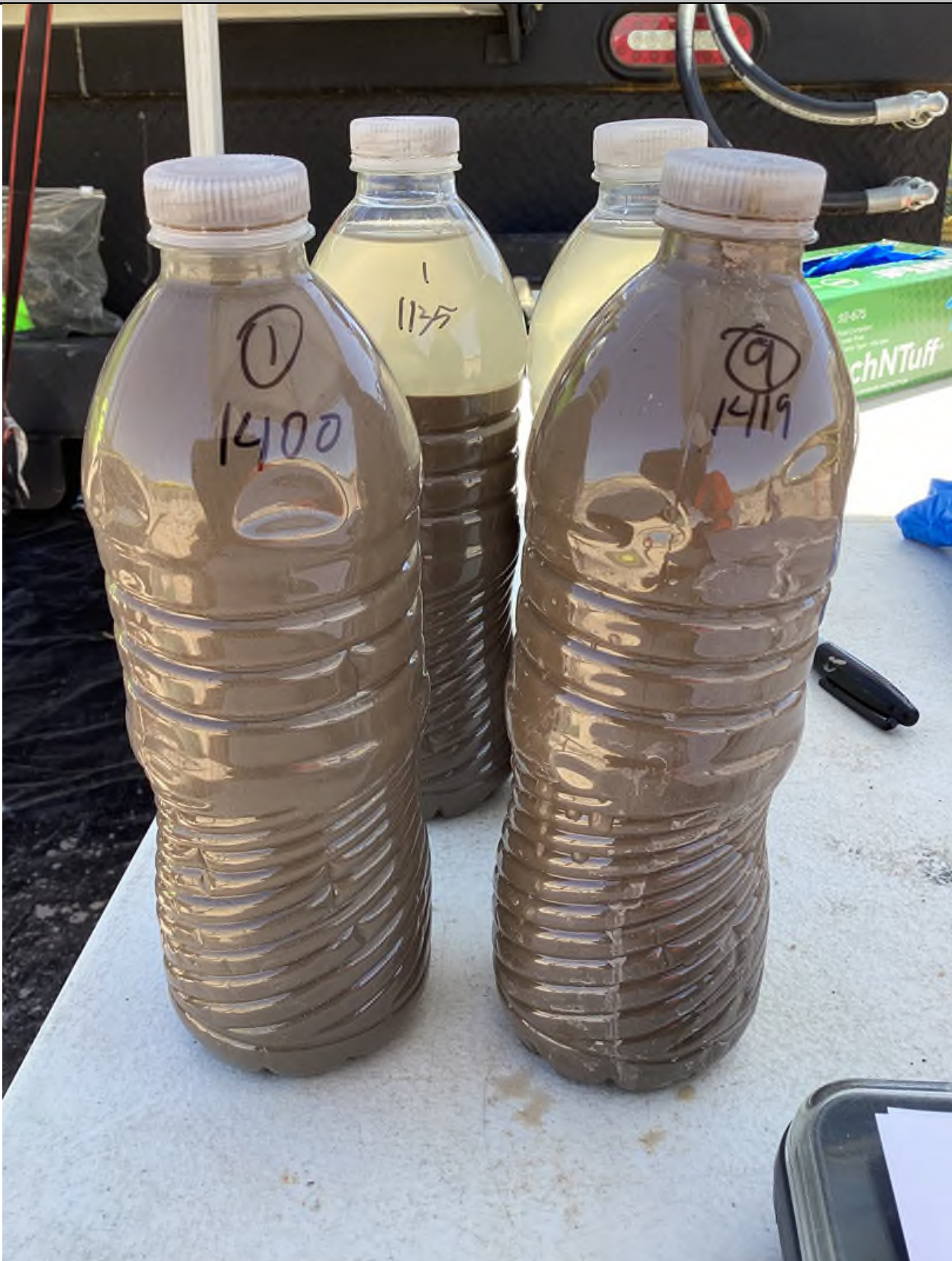
Results of third round of bailing on 5/11/2023. Left bottle shows first bailer removed and right bottle shows last bailer of the round which was the 9th bail. First redevelopment day.
