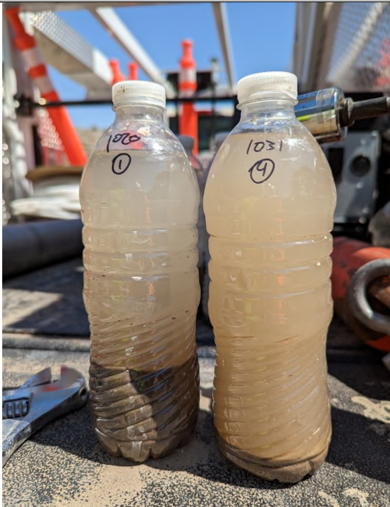
Results of second round of bailing. Left bottle shows first bailer removed and right bottle shows last bailer of the round which was the 4th bail.
