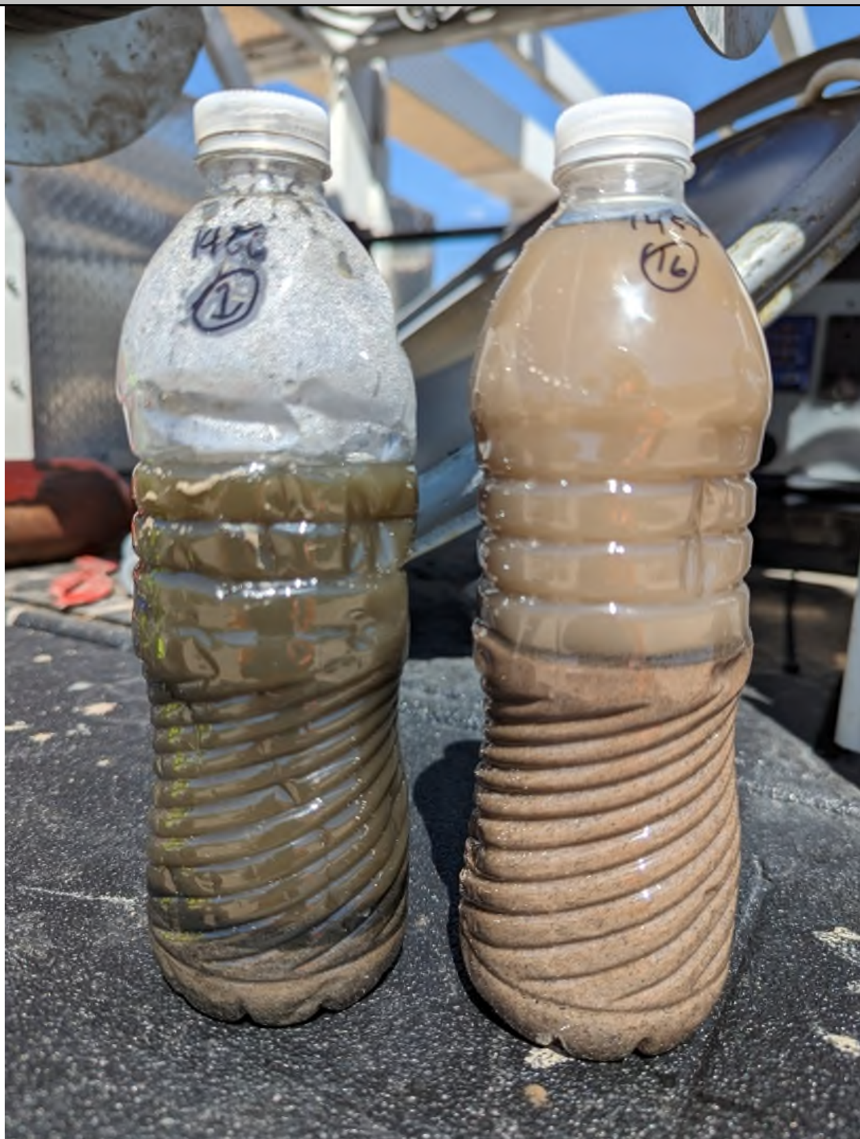
Results of first round of bailing, which occurred on 5/12/23. Left bottle shows first bailer removed and right bottle shows last bailer of the round which ended up being the 16th bail. First redevelopment day.
