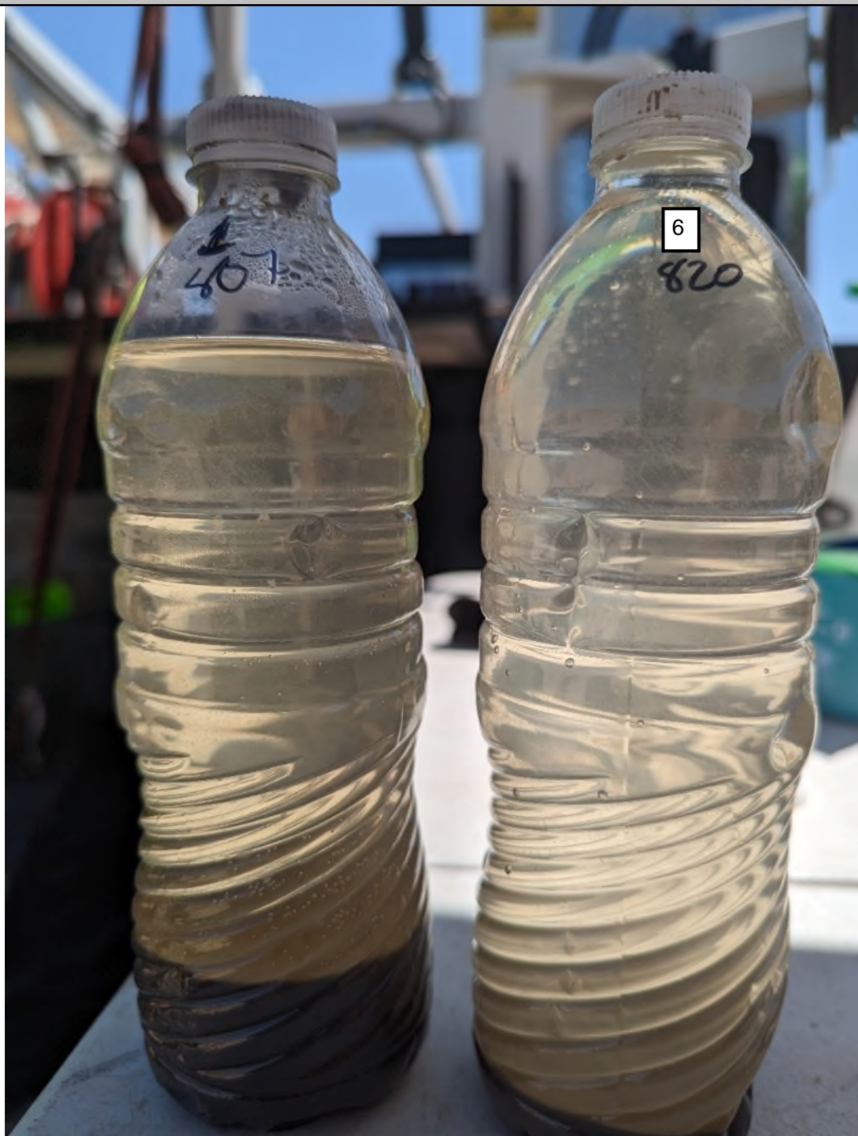
Additional photos of first round of bailing on 5/11/23. Left bottle shows first bailer removed and right bottle shows last bailer of the round which ended up being the 6th bail.
