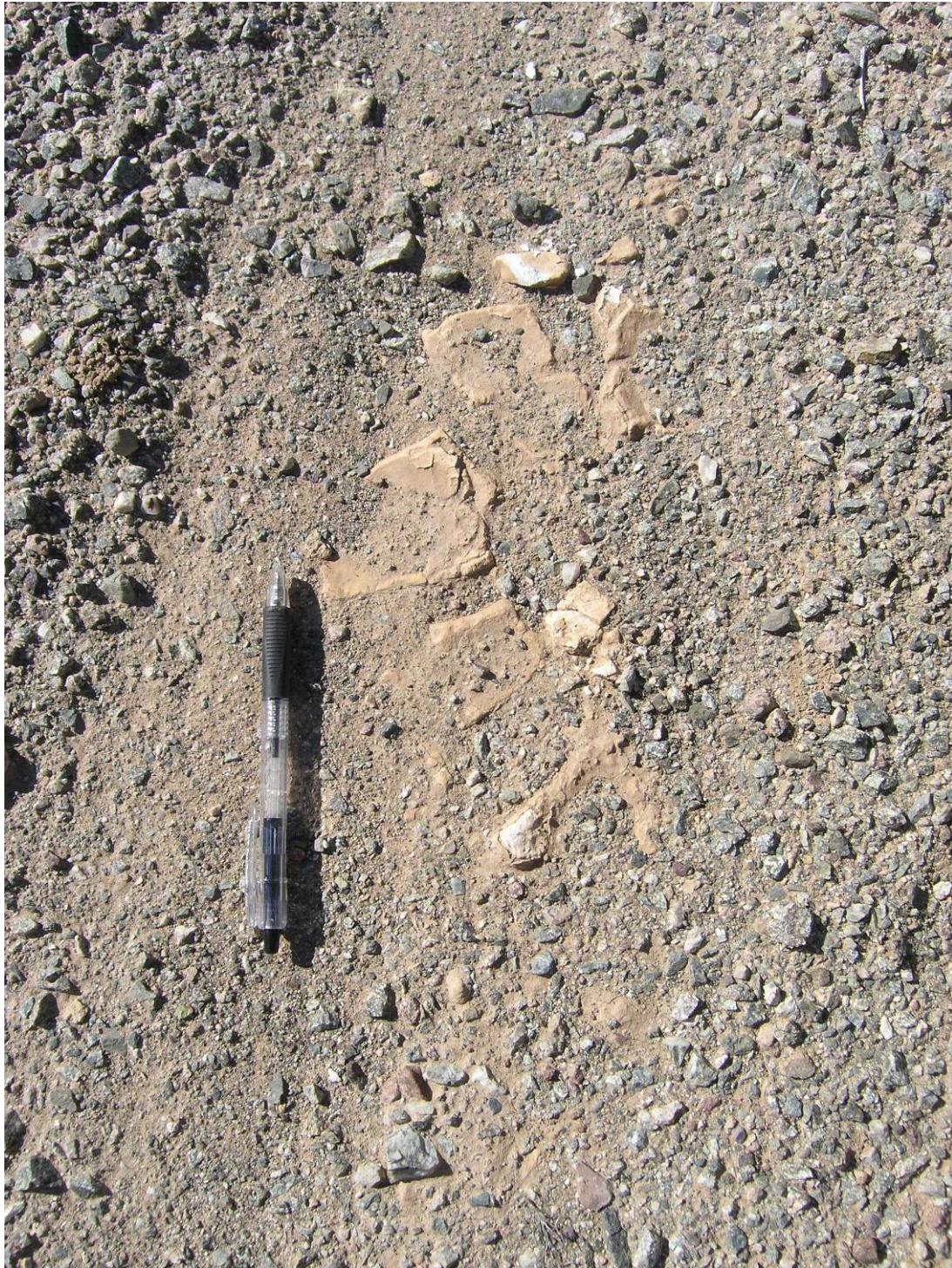
Figure 8. East Ravine. Close up of Figure 7 showing chunks of white powder at the surface of the wash (pen is 5.5 inches long). Sample DTSC AOC10d-3 area. The white powder was stained brown at its surface making the white material difficult to locate.
