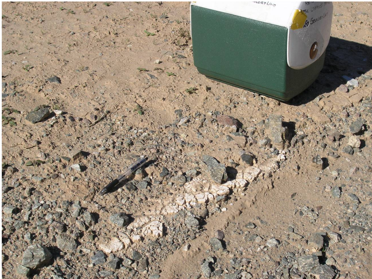
Figure 3. East Ravine. Close up of Figure 2. The white powder layer is approximately one quarter to one eighth inch thick. The pen is 5.5 inches long. Sample DTSC AOC10d-1 was collected from the white material only.
