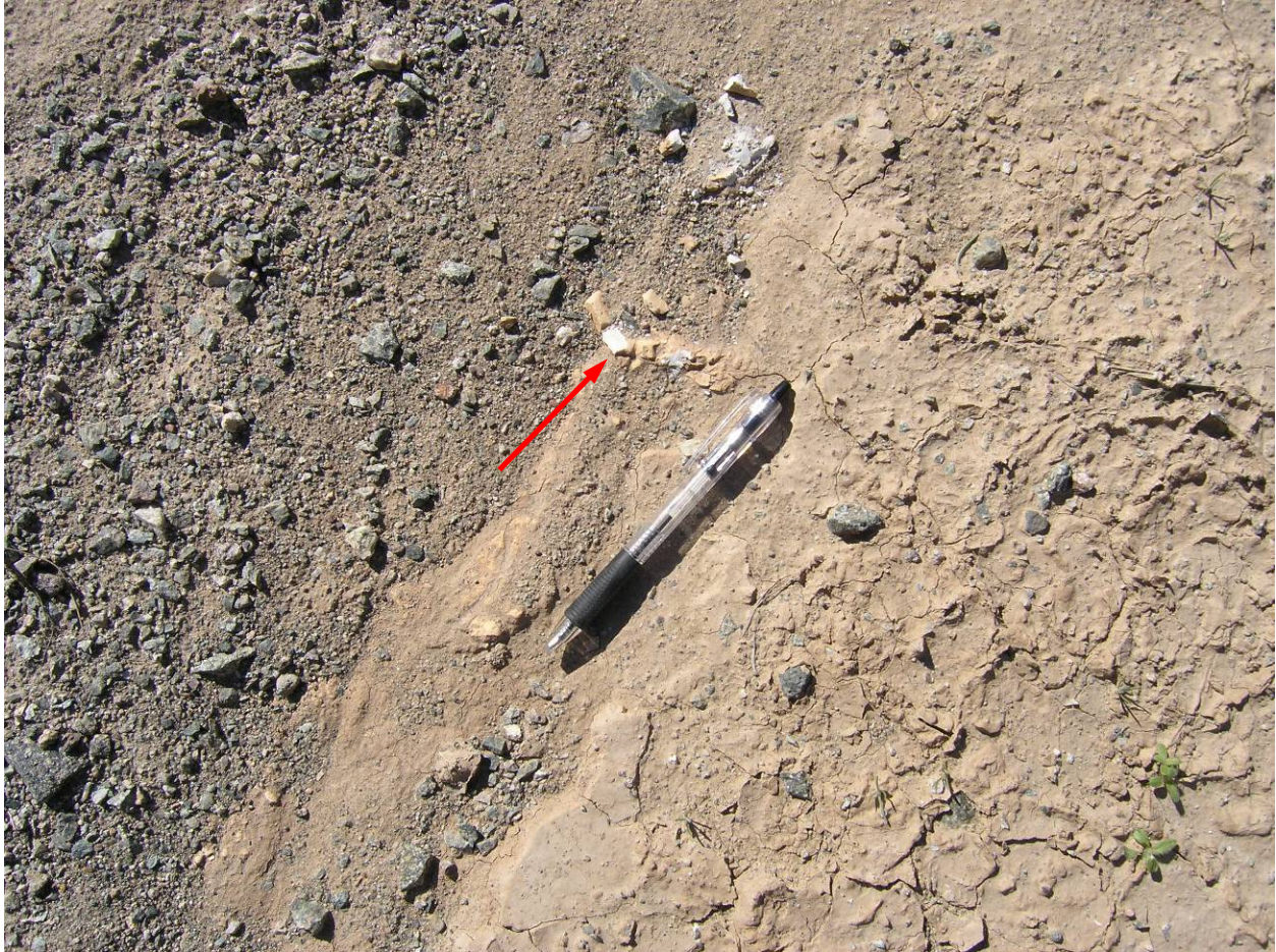
Figure 6. East Ravine. Close up of Figure 5 showing chunks of white powder at the surface of the wash (pen is 5.5 inches long). Sample DTSC AOC10d-2 area. The white powder was stained brown at its surface making the white material difficult to locate.
