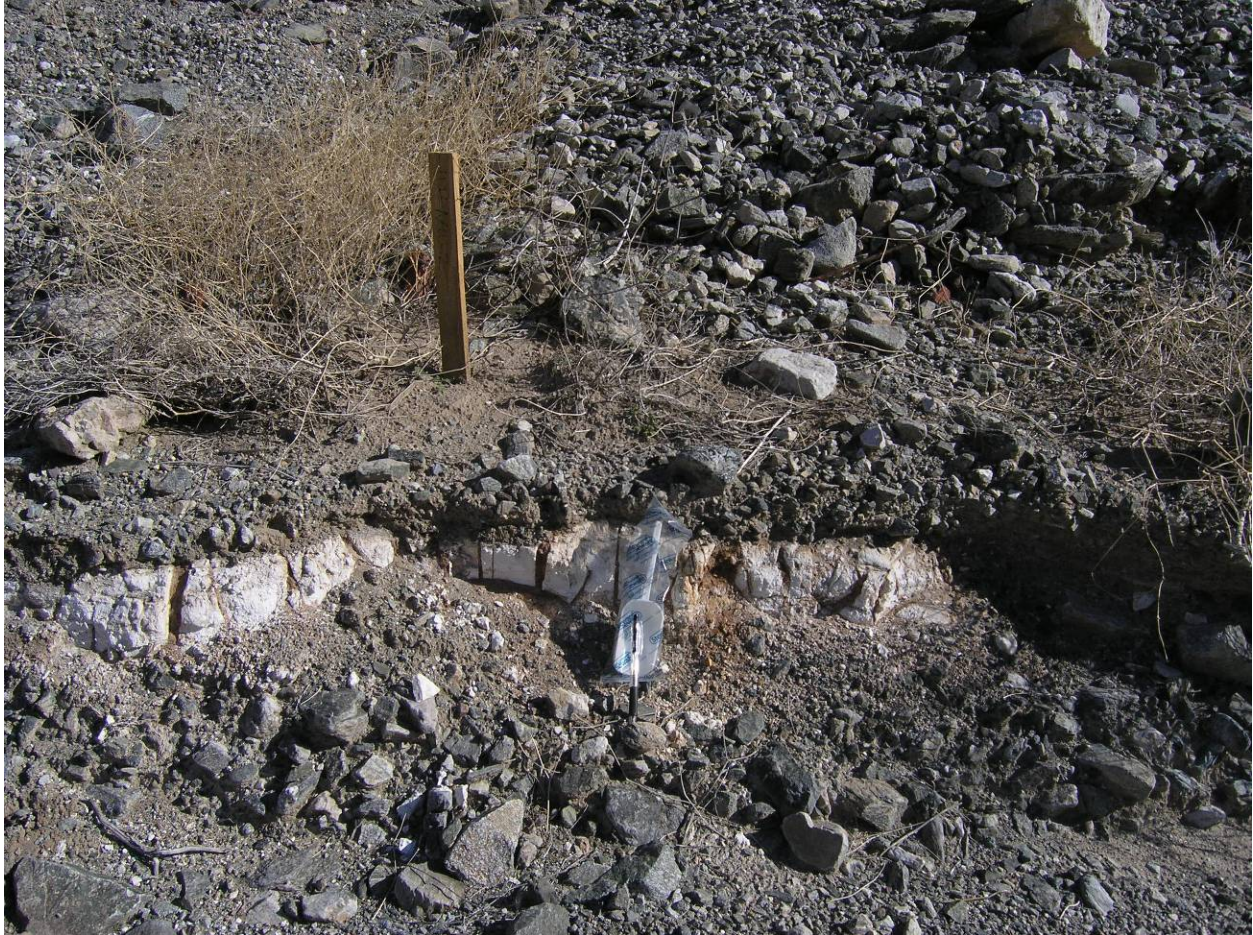
Figure 10. East side of Bat Cave Wash showing the white powder layer at the base of the wash (pen on top of plastic scoop is 5.5 inches long). The white layer is approximately three inches thick and large cracks in the layer are filled with dark reddish soil. Sample DTSC WP-NEW-2 area. The sample was collected from white material only. Note: PG&E's Part A soil sample stake in the background was labeled "WP-NEW-2".
