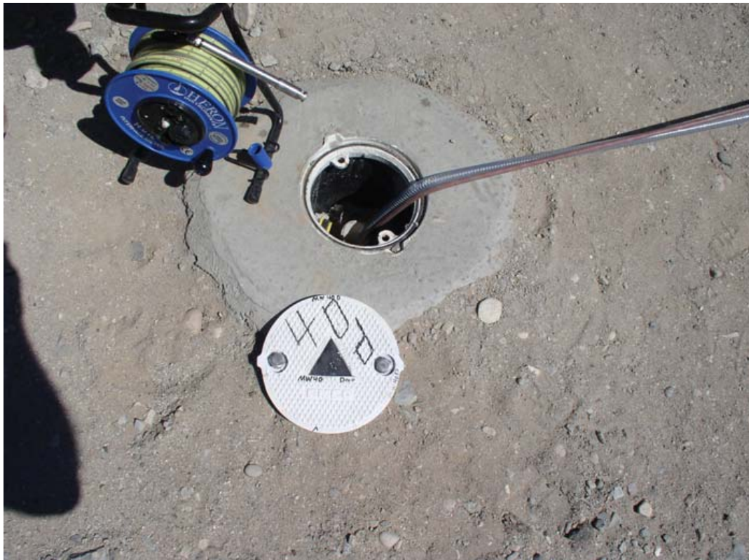
Typical monitoring well surface completion
