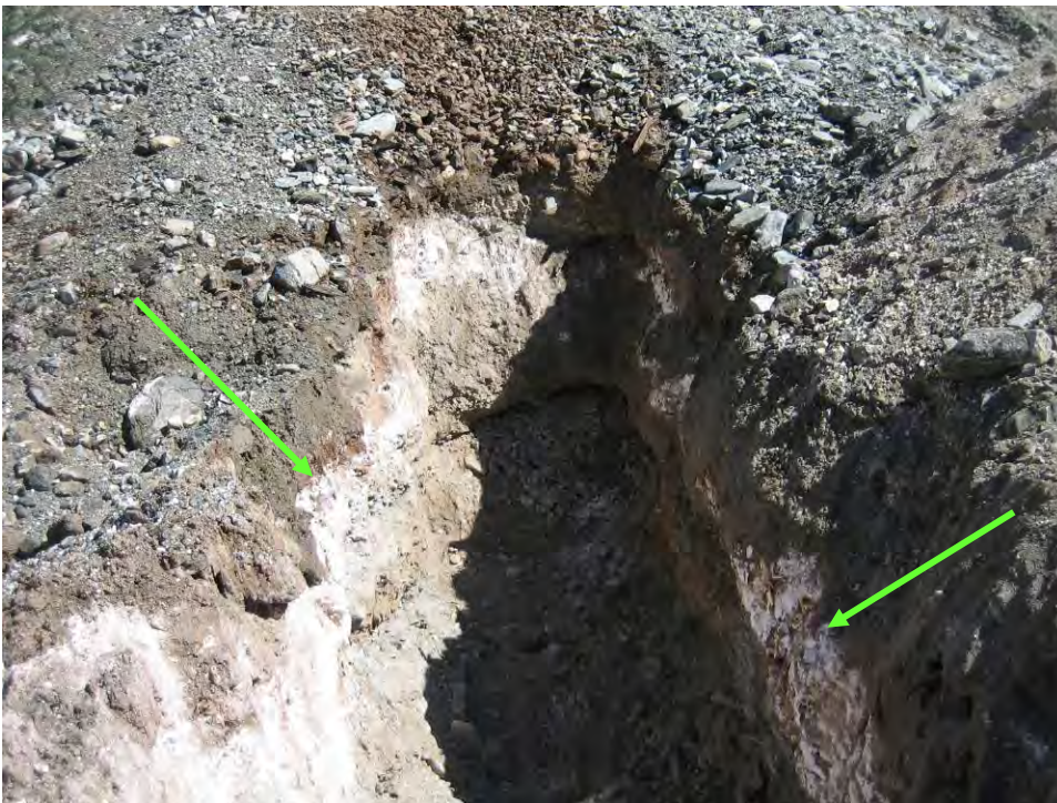
Photograph 18: Trench SWMU1-WP7 center. Note consolidated layer of white chalky material.
