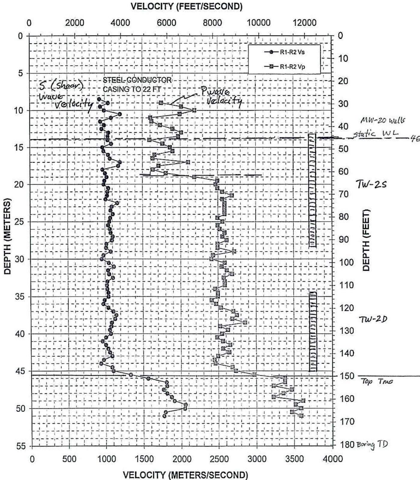
Figure 4: Borehole TW-2D, Suspension P- and S<sub>H</sub>-wave Velocities
