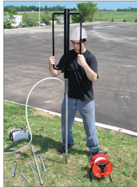
Installing Piezometers with a Manual Slide Hammer
