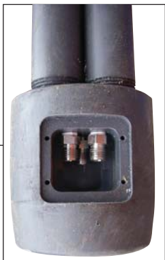
A. Transition centralizer attached to transducer pipes. Compression fittings for sample tubing exposed.
