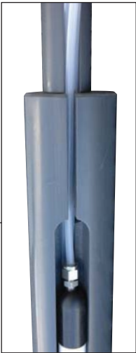
Top of sample filter in protective housing. Sample conveyance tubing attached and channeled in support riser recess.
