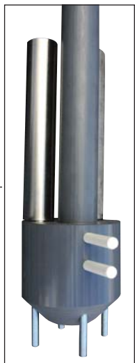
Anchor centralizer with left-hand threaded subs for tremie pipe and sounding conduit. White pins are driven into assembly to join.
