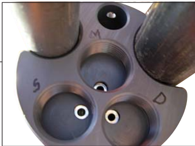
B. Top of transition centralizer without transducer pipes attached.
