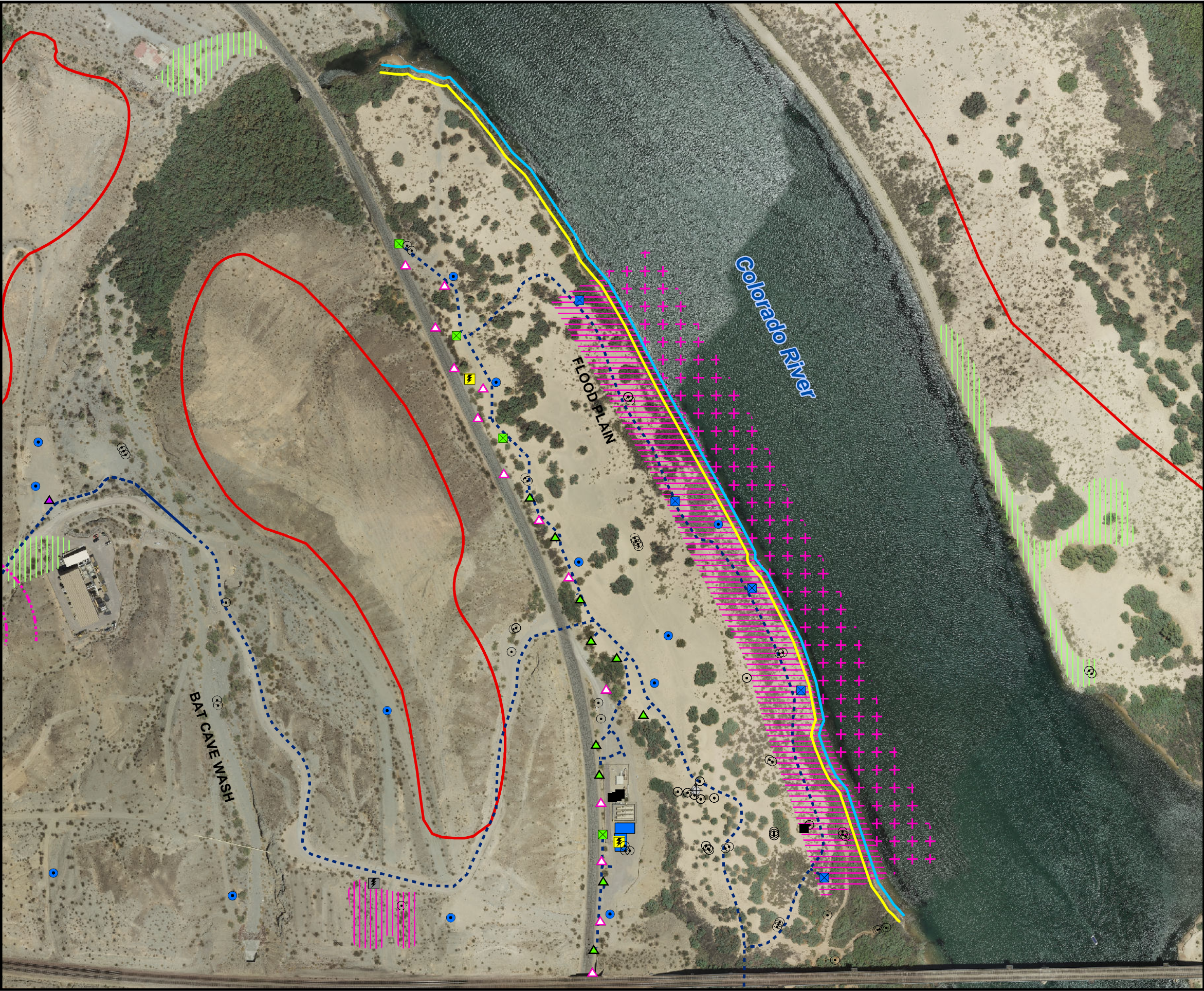
FIGURE 2.4-6 ORDINARY HIGH WATER MARK AND 20-FOOT SETBACK REQUIREMENTS ALONG RIVERBANK (EIR MITIGATION MEASURE AES-2A) GROUNDWATER REMEDY BASIS OF DESIGN REPORT PRE-FINAL (90%) DESIGN PG&E TOPOCK COMPRESSOR STATION, NEEDLES, CALIFORNIA
