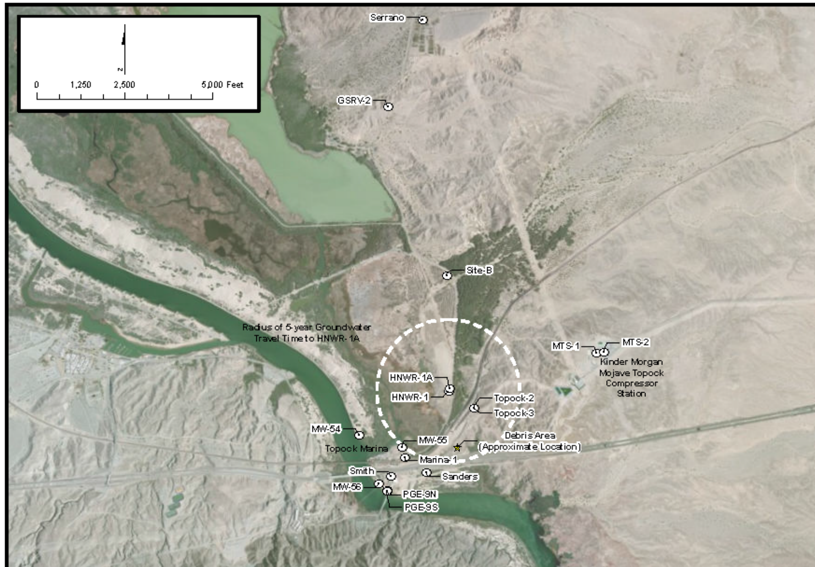
EXHIBIT 3.3-3 RADIUS OF FIVE-YEAR GROUNDWATER TRAVEL TIME TO HNWR-1A WELL Groundwater Remedy Basis of Design Report/Pre-Final (90%) Design PG&E Topock Compressor Station, Needles, California
