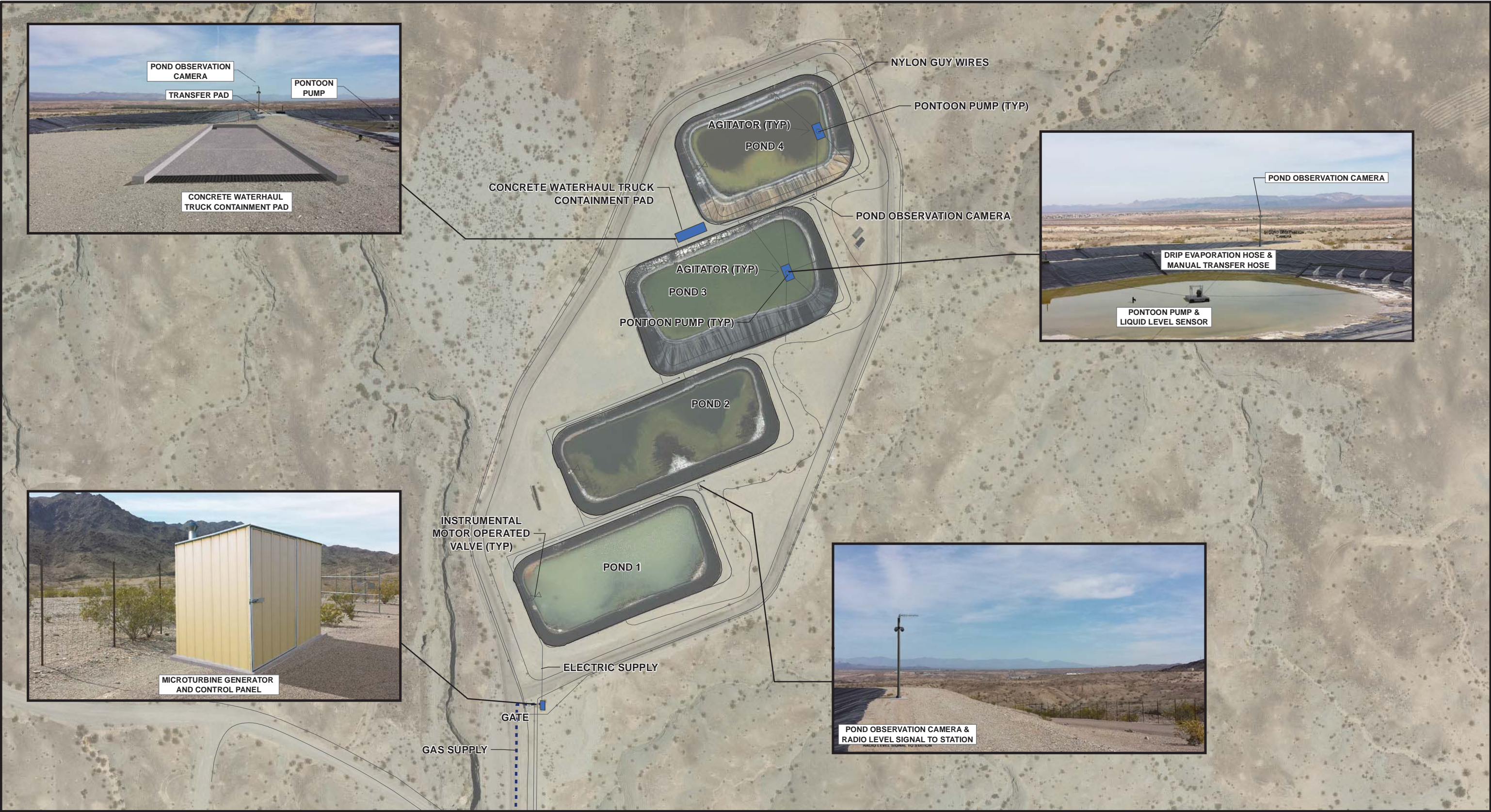
FIGURE 3.4-1 LAYOUT OF EVAPORATION ENHANCEMENT EQUIPMENT AT THE TCS EVAPORATION PONDS GROUNDWATER REMEDY BASIS OF DESIGN REPORT PRE-FINAL (90%) DESIGN PG&E TOPOCK COMPRESSOR STATION, NEEDLES, CALIFORNIA
