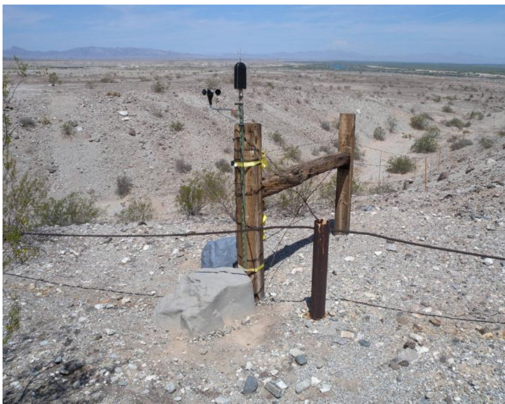
Photograph 2: Temporary Noise Monitoring Station set up in proximity to ST-1 noise measurement location in the certified EIR (DTSC, 2011), taken August 2012.
