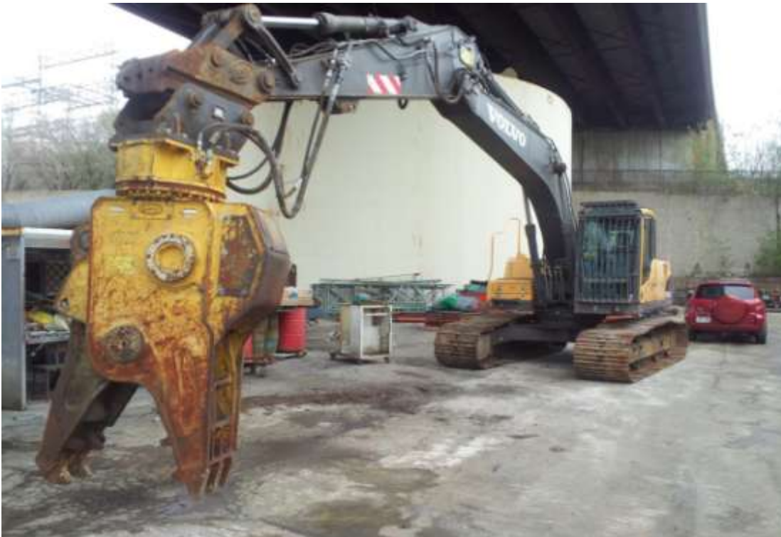
FIGURE 4-17 Typical excavator with pulverizer attachment
