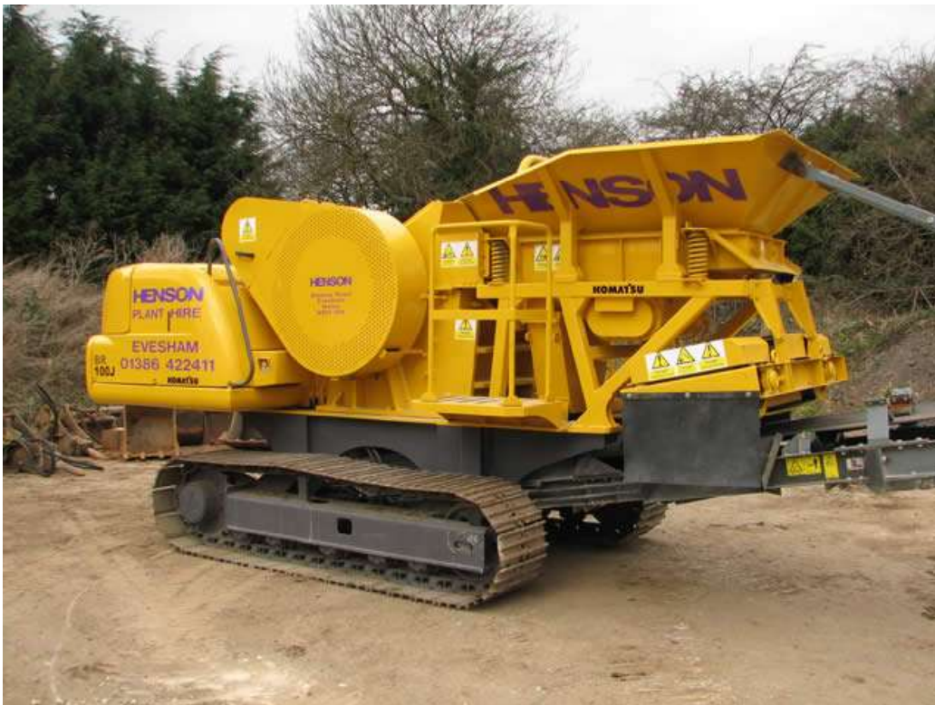
FIGURE 4-7 Typical concrete crusher
