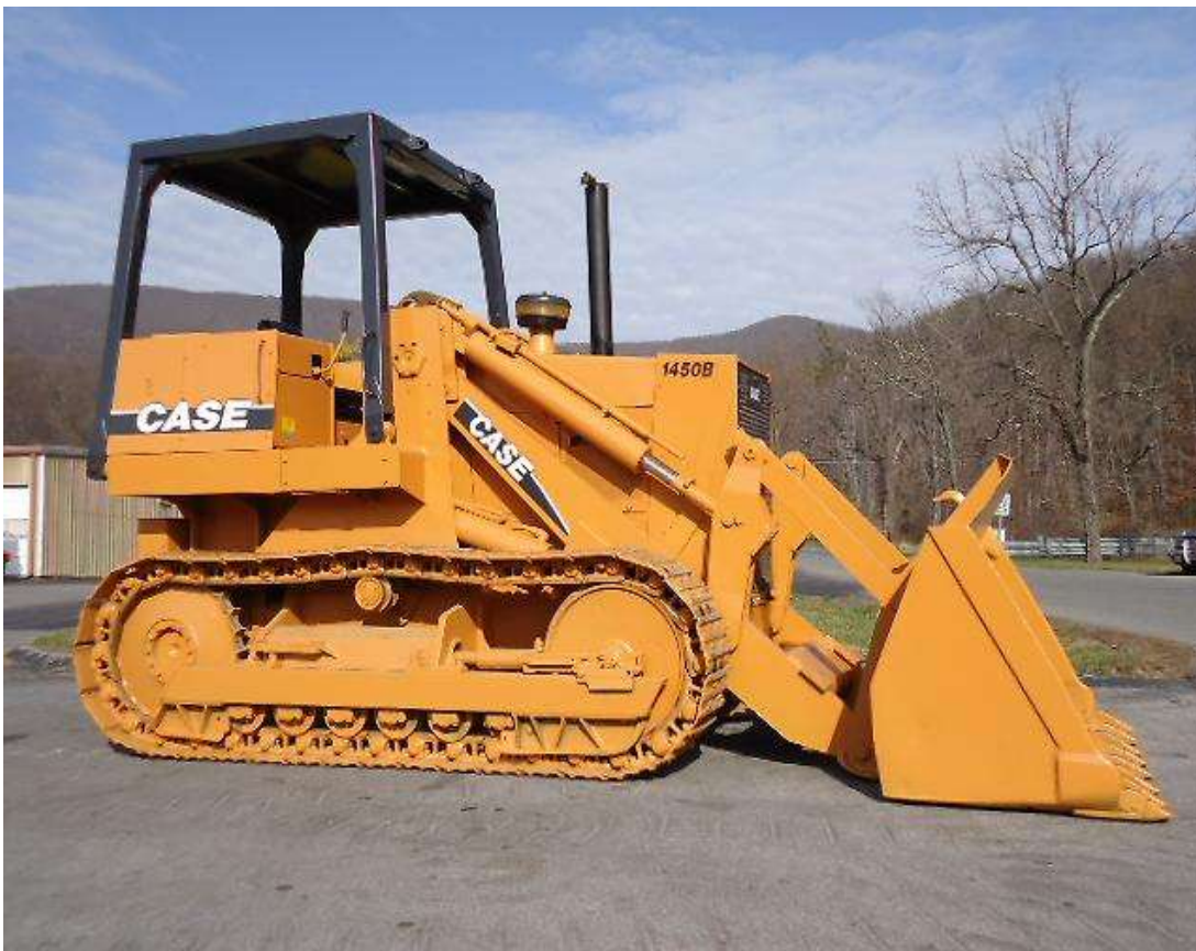
FIGURE 4-15 Typical front end crawler loader
