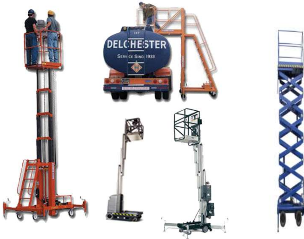
FIGURE 4-20 Typical personnel lifts (left), scissor lift (right)
