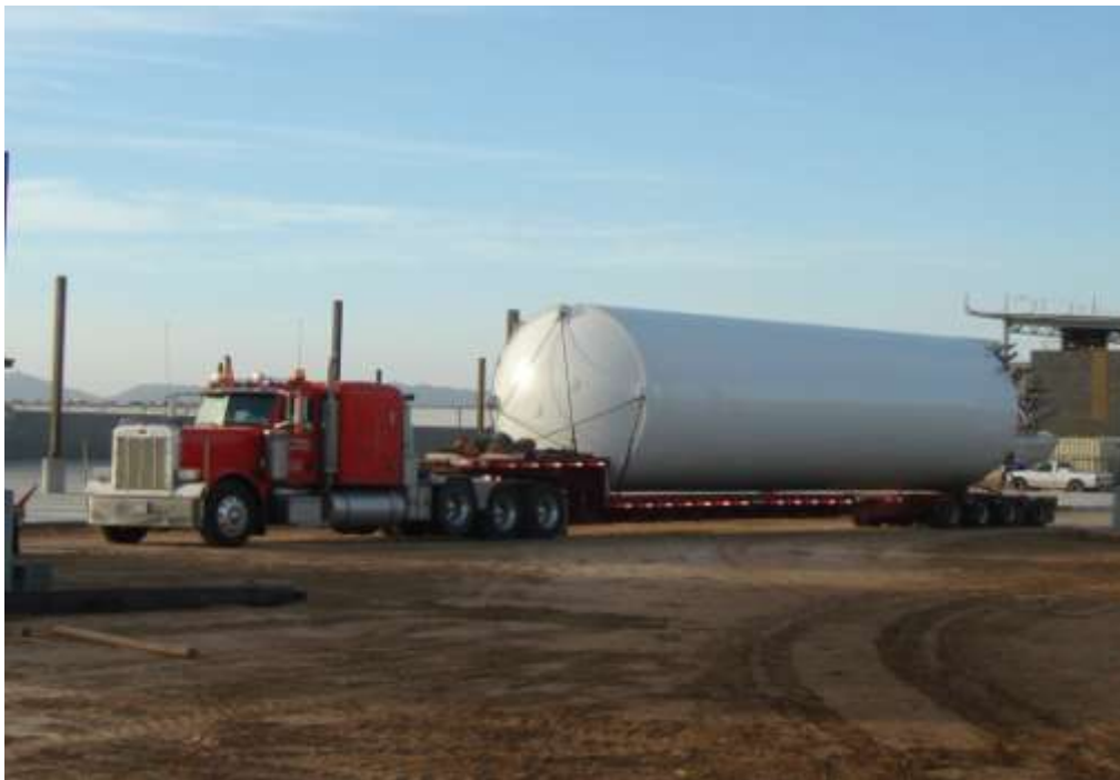
FIGURE 4-5 18-Wheeler with flatbed trailer showing tank removal
