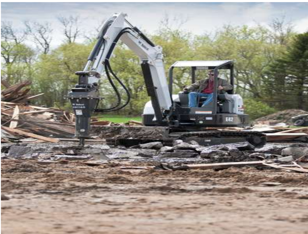
FIGURE 4-23 Typical compact excavator with breaker attachment
