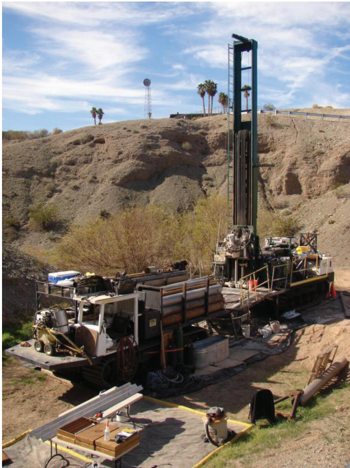
Example of a Track-Mounted Rotosonic Drill Rig and Support Vehicle Used for Locations with Difficult Access
