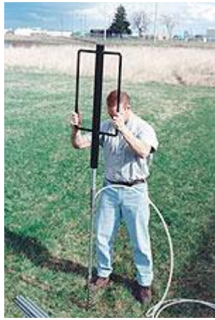
Installing a drive-point piezometer with a manual hammer.
